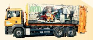
The collection truck remains in its area of deployment and simply swaps its full transport container for an emptied transport container at an intended location.
