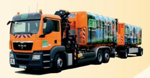
The full interchangeable container is transported together with another full interchangeable container on a bulk tipper to the waste disposal plant for emptying. We implement this transport system across the district for the collection of residual waste and cardboard/paper.
